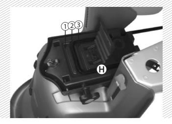
In order to adjust the baby seat onto the bicycle, put the metallic rod into one of the three allowed positions.
