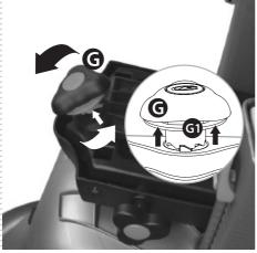
Unscrew the hand knob (G) and simultaneously lift the red security ring (G1).
