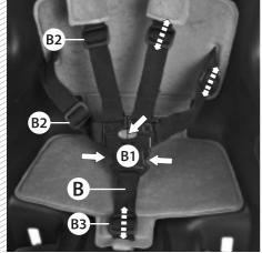
To put the child in the seat, open the lock (B1) of the safety belt (B) and press the three buttons of the lock (B1) as indicated. Before starting your ride, make sure the seat belt is properly adjusted and that it does not hurt the child. This adjustment is made by sliding the belt adjustors (B2) and (B3).
