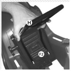
Hold the metallic bracket (H) the same as in the picture and pass it through the opening in the baby seat.
