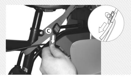
Pass the safety belt (C) around the bicycle frame. Adjust it as shown in the picture, under tension.
