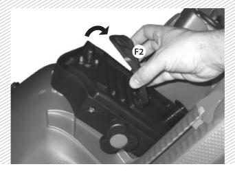
Rotate the plastic mounting plate (F2).
