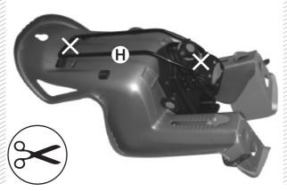
Remove the metallic bracket (H) from the seat by cutting the straps.
